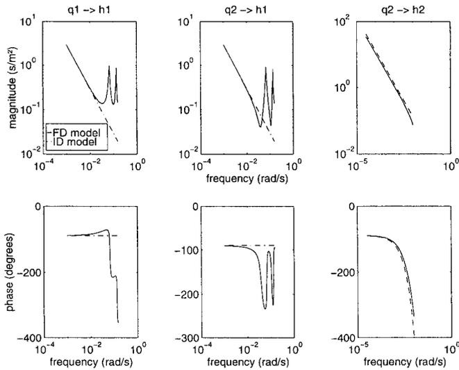
FIG. 5. Bode Diagrams of Test Canal One
