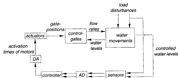
FIG. 1. Block-Diagram Showing Some of Most Important Processes in Controlled Canal
