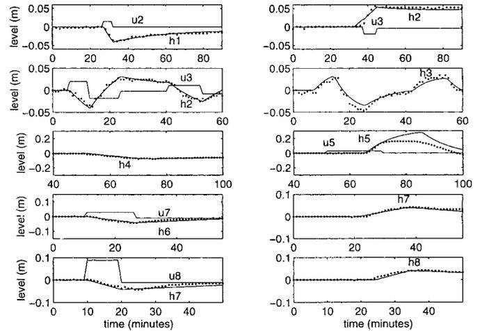
FIG. 7. Water Level Variations ( $h_1$ – $h_8$ ) in Response to Gate Opening Variations ( $u_1$ – $u_8$ ). Solid Line: Simulated Levels; Dots: Measured Levels
